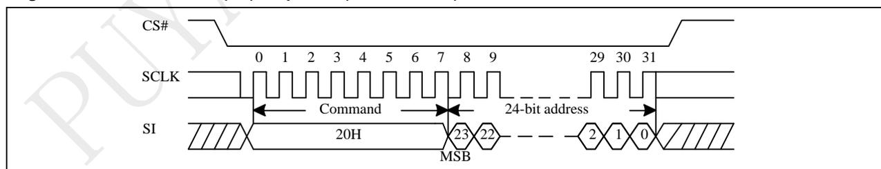
The self-timed Sector Erase Cycle time ( $t_{SE}$ ) is initiated as soon as Chip Select (CS#) goes high. The Write in progress (WIP) bit still can be checked out during the Sector Erase cycle is in progress. The WIP sets 1 during the  $t_{SE}$  timing, and sets 0 when Sector Erase Cycle is completed, and the Write Enable Latch (WEL) bit is reset. If the sector is protected by BP4, BP3, BP2, BP1, BP0 bits, the Sector Erase (SE) instruction will not be executed on the sector.
