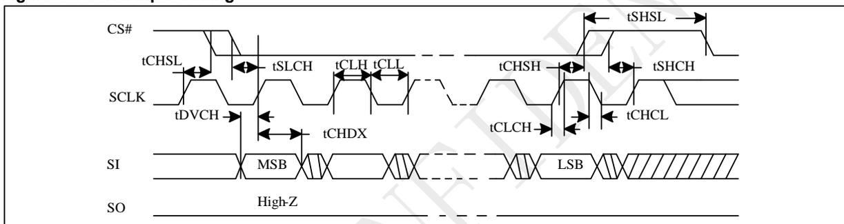
Figure 5-5 Output Timing
